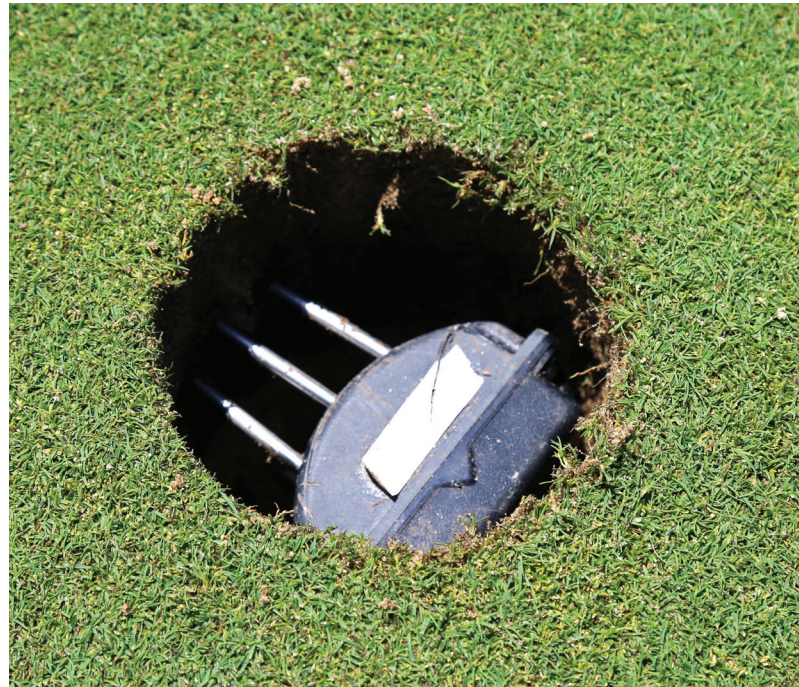
In-ground soil-moisture sensors help superintendents track moisture trends and identify thresholds for irrigation.
