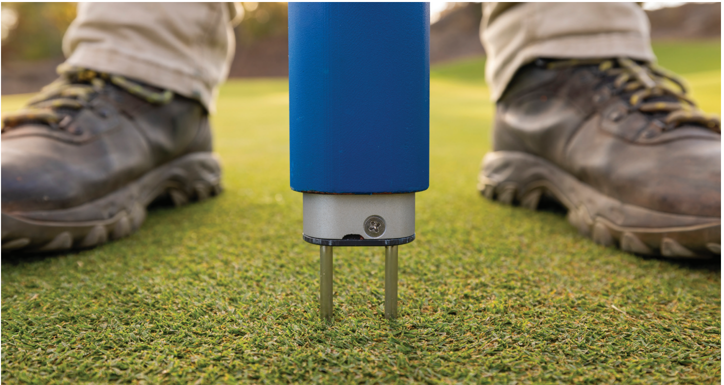
Using technology like soil-moisture sensors can give superintendents a better understanding of turfgrass water needs throughout a golf course. (USGA/Kyle LaFerriere)
