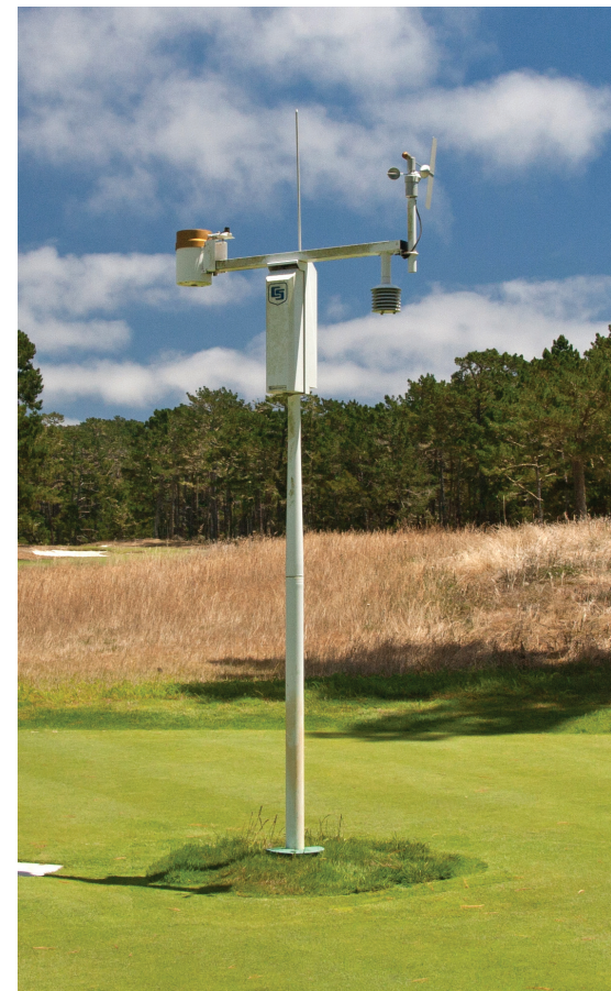
An on-site weather station is the best way to obtain ET data that is site-specific to a particular golf course.
